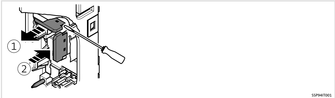
Fig. 4-12 Plugging the IT insulating cap onto the earthing jumper
